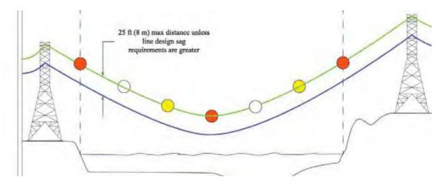
Fig. 4: A diagram of unlit marking balls.<sup>7</sup>
