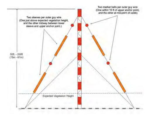
Fig. 3: A diagram of marking of a tower.<sup>6</sup>
